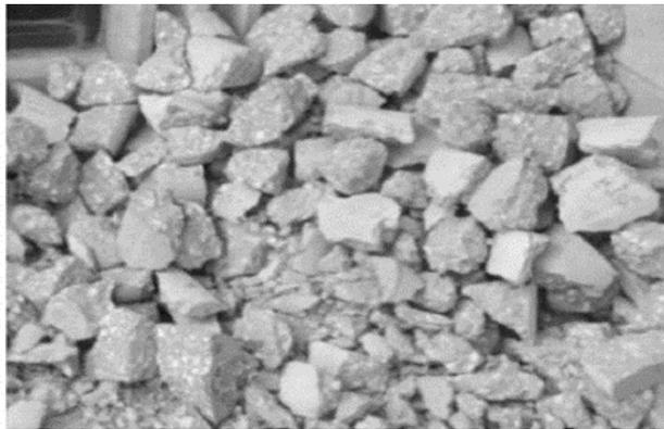
Figure 2. Recycled Concrete Cubes and Cylinders Used
